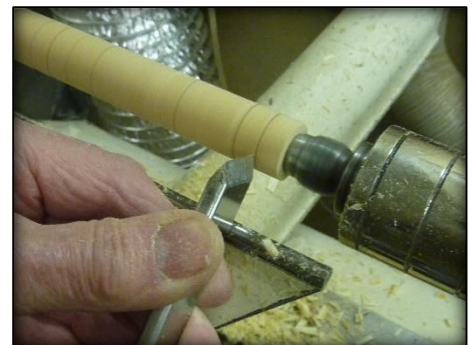
#6 Frontal view of cut with the toe of the skew
