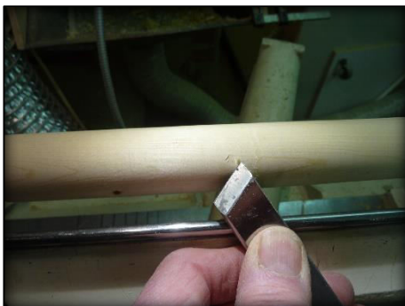
#4 Planing cut showing toe getting too low and catch happens
