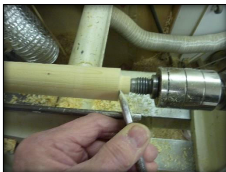
#8 Squaring off with toe of the skew. Note, leave slight angle away from the cut to avoid catches, but, bevel rubbing at the toe
