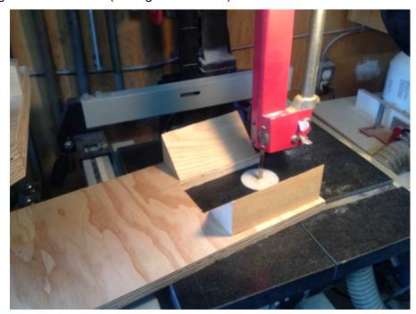
• Placing the bowl blank in the slot, hold the blank on the sides (not the end) and line up the centre line on the spacer board with the bandsaw blade. Slowly cut the two halves apart, by sliding the jig forward through the blade.
