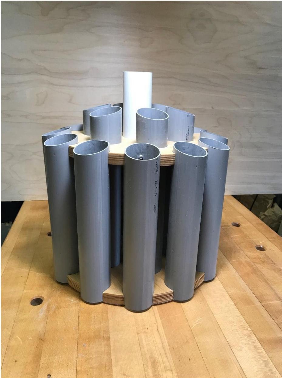
*Figure 1 Note the screw placement in the top of the tubes and the fact that the bottom of the tubes are "captured" in the plywood disc.*
