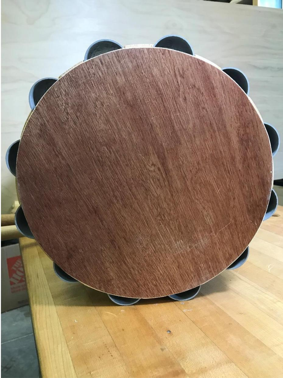
*Figure 1 This photo shows the relative sizing of the underlayment and the tube placement allowing dust to escape from the tubes. The center tubes will require a vacuum to clean them, if needed.*
