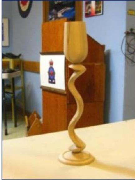
**Purpose:** To produce a wavy candlestick using parallel axis turning.
