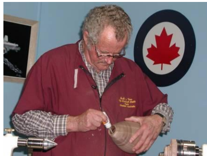
Preparing his bottom plug hole, using CA glue
